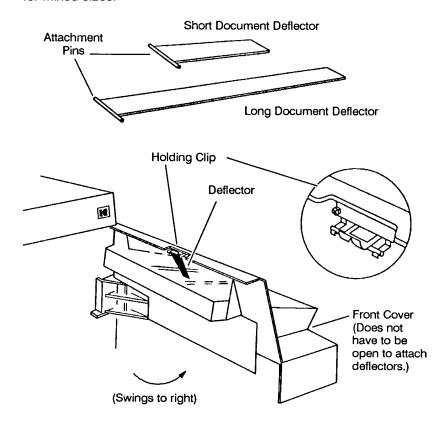
Grasp the deflector near the attachment pin (as shown).
